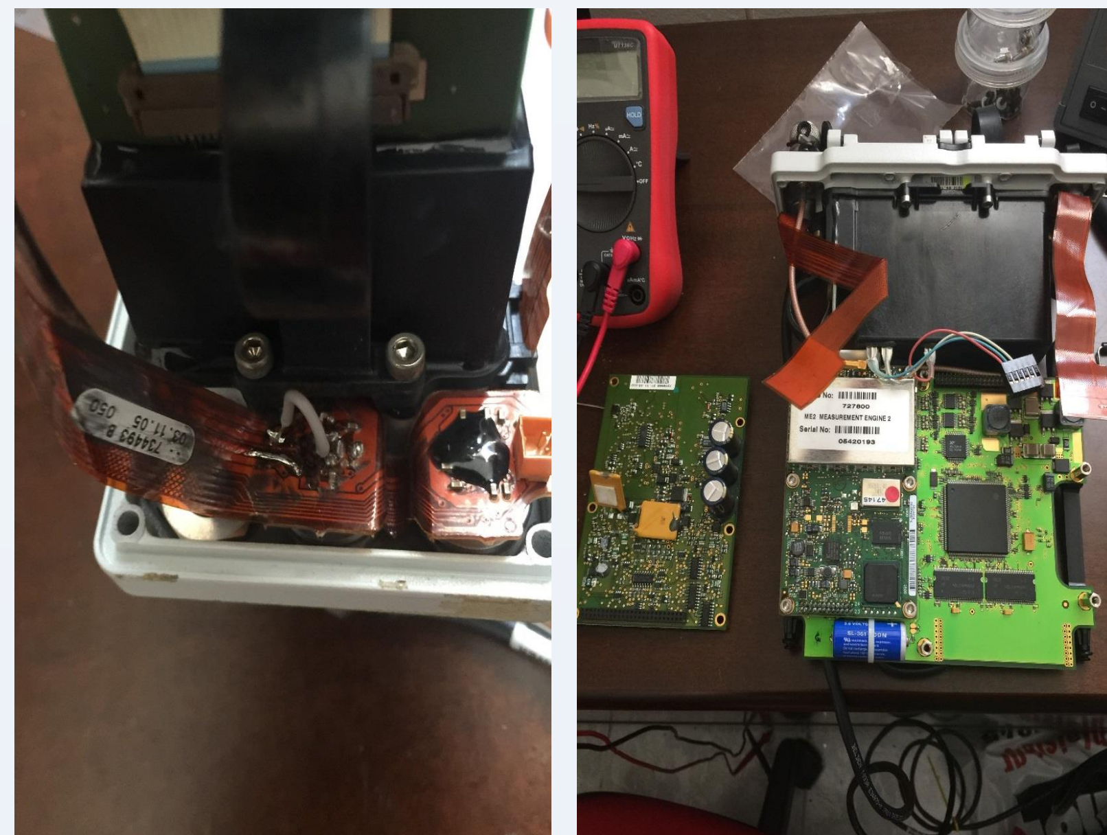
Fig.1 GNSS receiver unit damage from surge voltage
