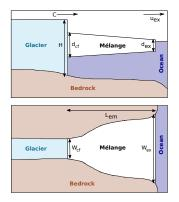
Geometry of the glacier terminus, ice mélange and embayment as a side view and a top view. The side view shows the ice thickness H, the calving front thickness  $d_{cf}$  and exit thickness  $d_{ex}$  of the ice mélange as well as the calving rate C and the mélange exit velocity  $u_{ex}$ . The top view shows the embayment width at the calving front  $W_{cf}$  and the embayment  $L_{em}$ .
