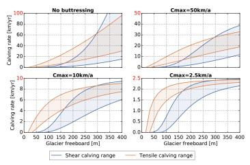
Calving rates as a function of glacier freeboard (ice thickness - water depth) in the unbuttressed case and for a range of upper bounds  $C_{max}$ . Shear calving and tensile calving rates depend also on the water depth: Two lines are shown for each configuration, the lower line for a dry cliff (w = 0.0) and the upper line for a cliff at floatation (w = 0.8). This spans the range of possible calving rates for a given freeboard.
