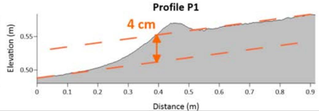
In order to accurately quantify the deformation of the ground surface, we surveyed the best locations with a terrestrial laser scanner (Faro), which allowed estimating a vertical uplift of the SE compartment comprised between 2.7 and 13 cm
