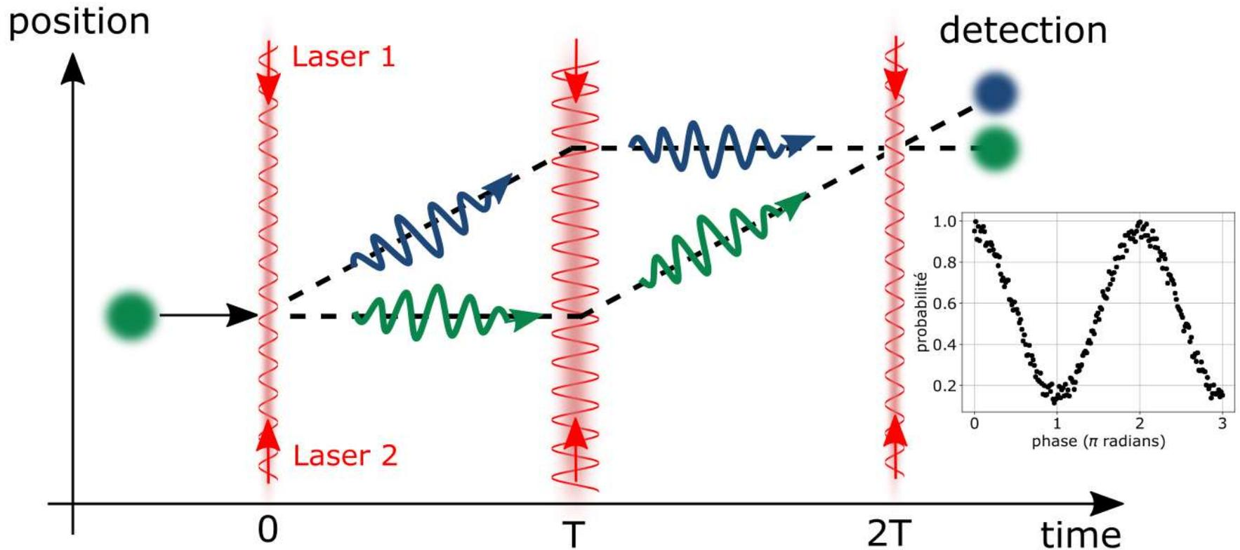
Two-wave interference signal :  $P = P_0 + A \cos(\Delta\Phi)$
