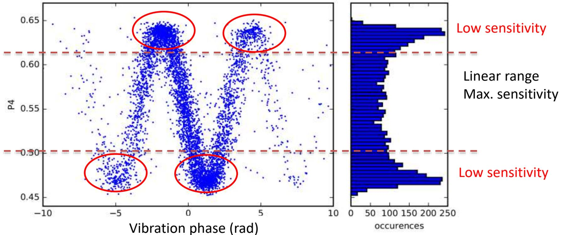
Real-time calculation of the vibration-induced phase (at each shot)
