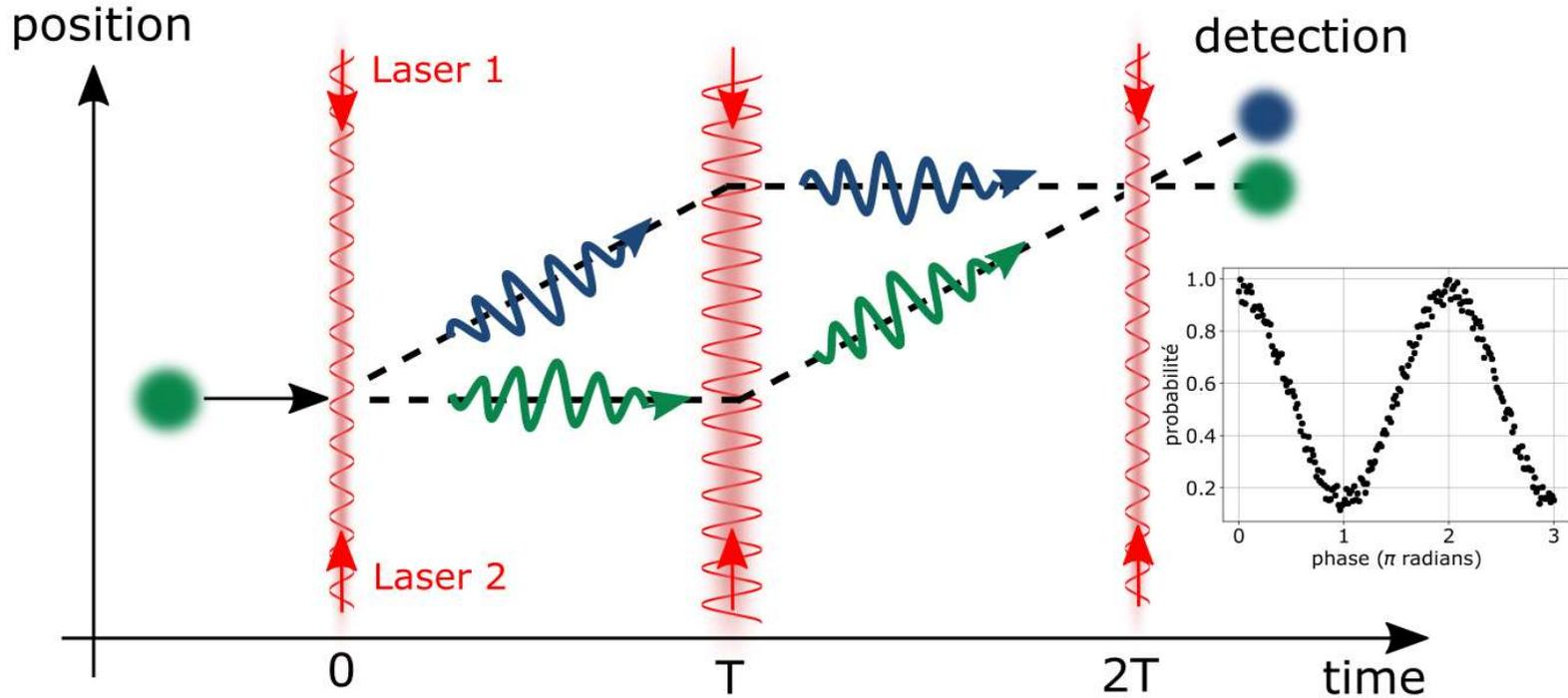
$$\Phi = \phi(0) - 2\phi(T) + \phi(2T) = \vec{k}_{eff} \vec{a} T^2 + 2\vec{k}_{eff} (\vec{v} \times \vec{\Omega}) T^2$$
