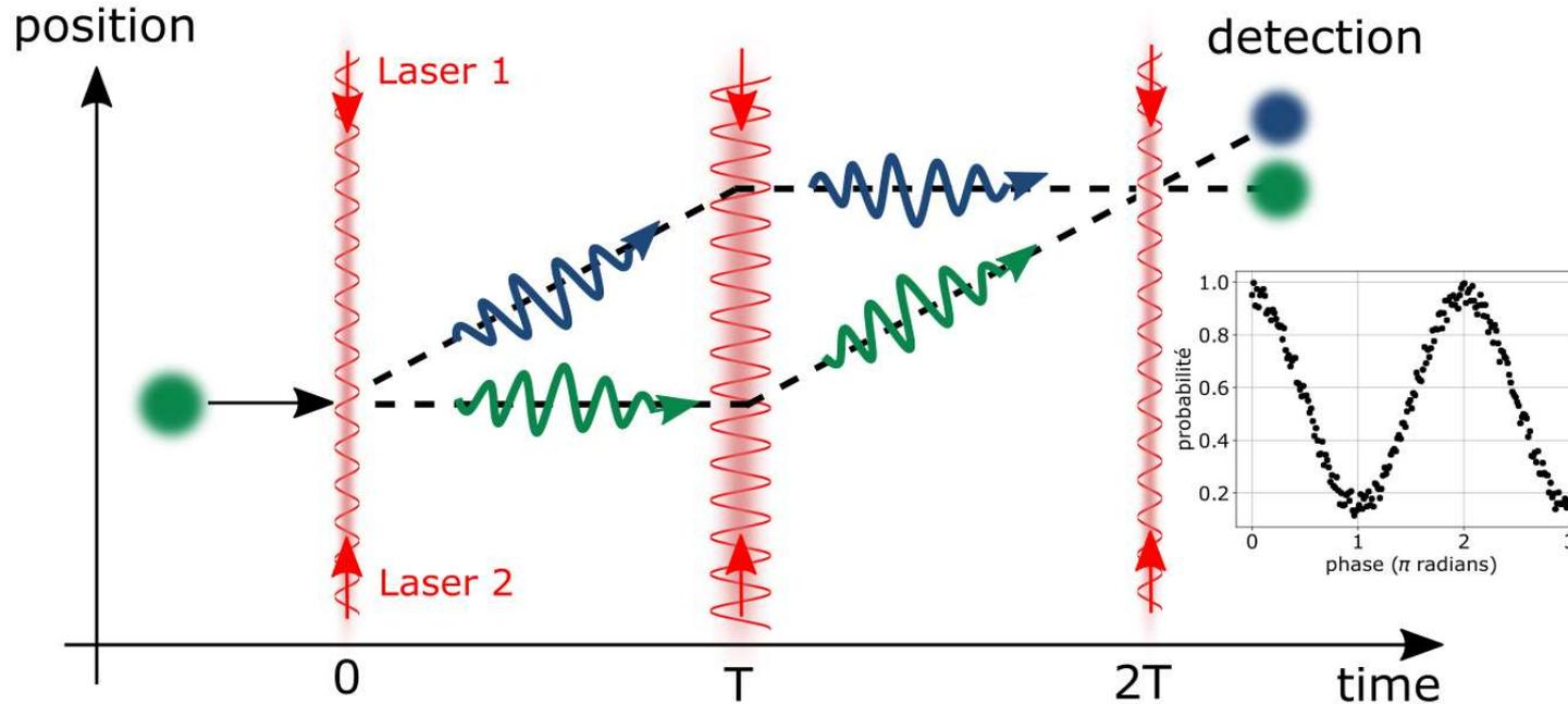
$$\begin{aligned} \text{Top path : } & \varphi(0) - \varphi(T) \\ \text{Bottom path : } & \varphi(T) - \varphi(2T) \end{aligned} \quad \longrightarrow \quad \Delta\Phi = \varphi(0) - 2\varphi(T) + \varphi(2T) = \frac{4\pi g T^2}{\lambda}$$
