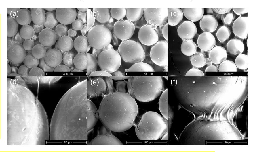
During drying mucilage forms liquid bridges between particles
