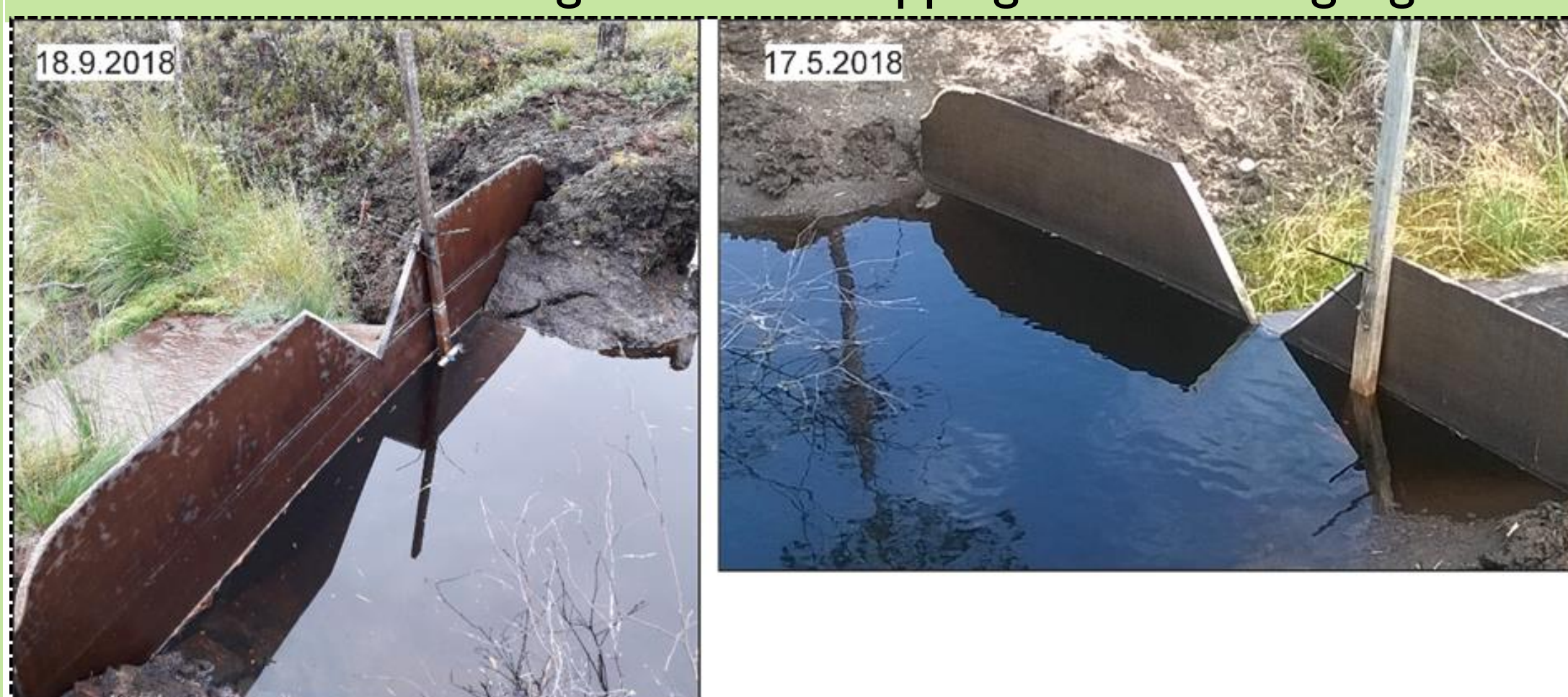
Runoff monitoring V-notch weir at the study site
