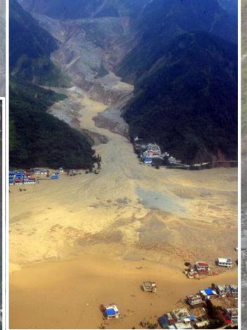
The 2010 Qingping debris flow deposited an estimated  $5x10^{-2}$  km<sup>3</sup> into the Min Jiang, (Tang et al 2012)
