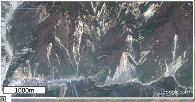
Using the inventory we were able to identify and quantify **2 temporary sediment stores** and **8 sediment transport** processes. We combined these with a further **3 processes** with estimates from the literature to complete the sediment budget
