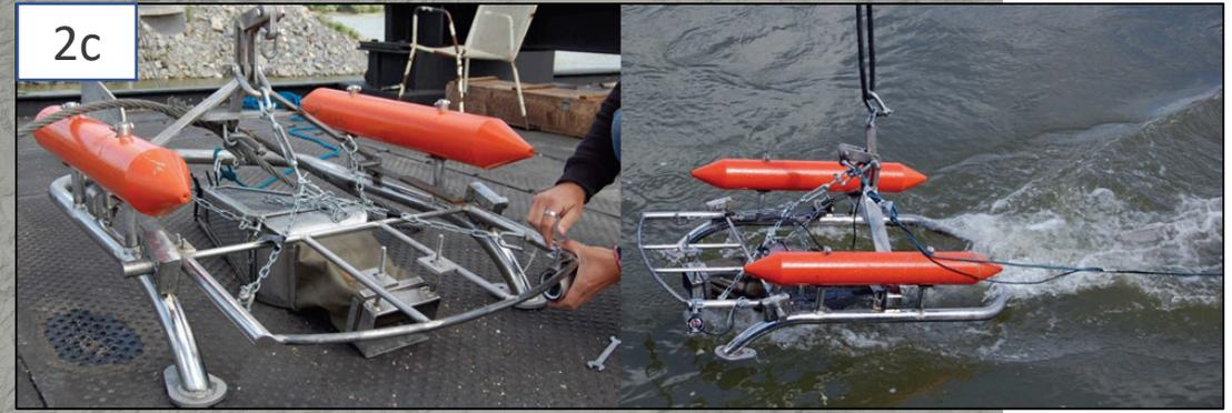
Figure 2a: sampling locations. 2b: example of picture for GSD data collection for the 2018 campaign. 2c: BFG basket sampler used by Hauer et al, 2019 at Pocem
