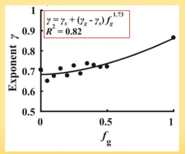
Via revised sediment transport formulae in both current-and wavedriven models (McCarron et al., in prep): effect of this newly quantified HE correction is greatest for gravel percentages between 10 and 20%.
