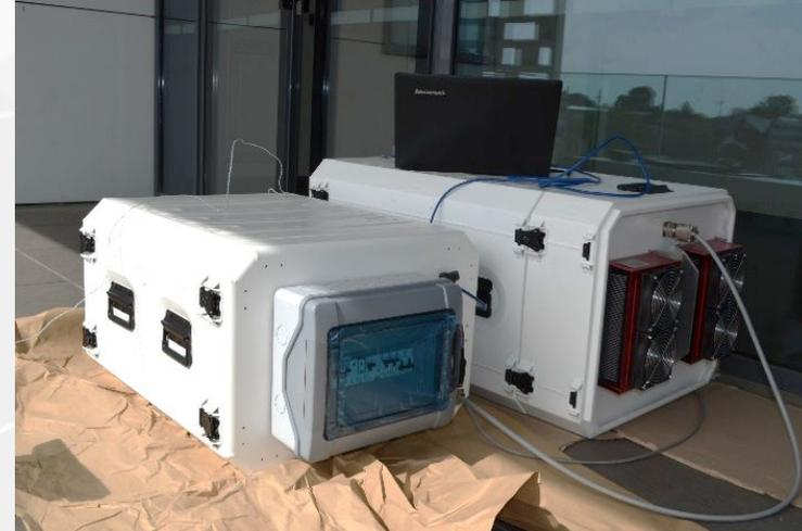
*AQG laser system operating outdoor, at a temperature of 38°C*
