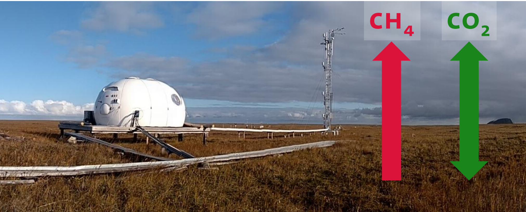
Vertical C fluxes of CO_2 and CH_4 were observed at the eddy covariance tower located within the catchment A.
