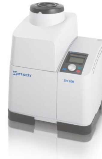
6. Retsch Ultra Centrifugal Mill ZM 200
