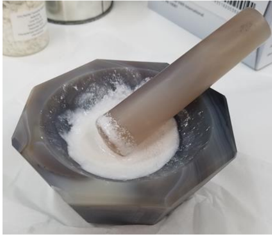
1. Hand Grinding using Agate Mortar/Pestle (With DI water)
