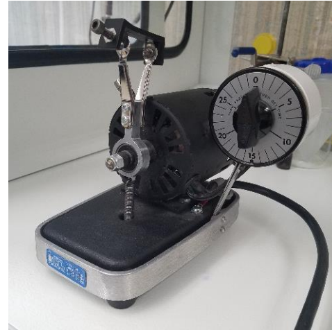
2. Impact Milling using a Ball Mill (Wig-L-Bug amalgamator)
