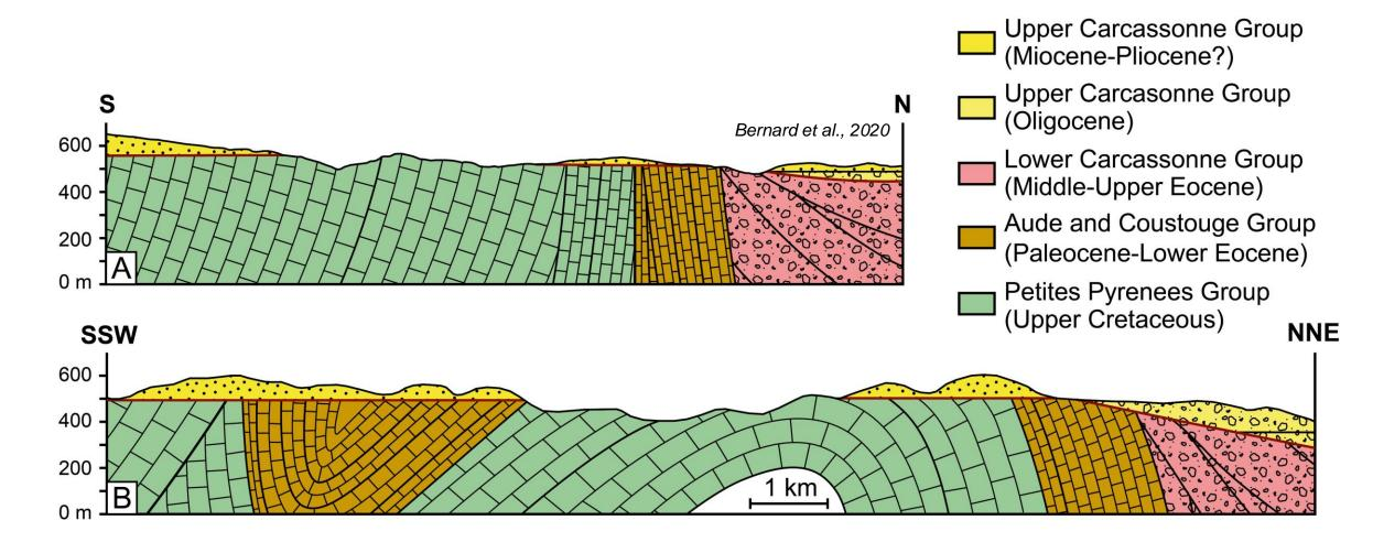
• Example of geologic cross-section in the Northern Pyrenees highlighting the drape and seal of syn-orogenic structures of the thrust-wedge by post-orogenic structures (Miocene Upper Carcassonne Group)
