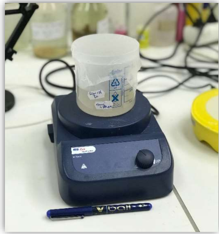
A batch trial on magnetic agitator
