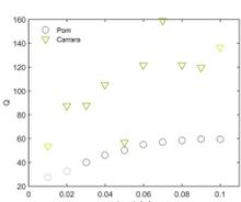
Figure 4: Results for Q from spectral ratio technique (with aluminum as reference) and different length for frequency range between 0.5 MHz and 0.8 MHz based on eq. (1) (Toksoz et al., 1979).
