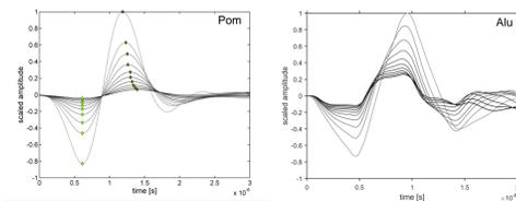
Figure 2: Example of first arrivals of Pom (left) and Alu (right) samples corrected for their phase travel times. Light and dark green diamonds (left) indicate first minima and first maxima, respectively. Amplitude scales to absolute maximum in the shown time interval.
