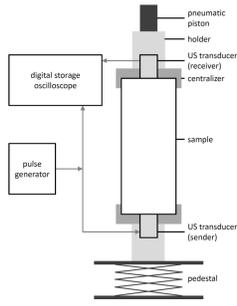
Figure 1: Experimental setup for ultrasound transmission. Reproducibility for travel times and amplitudes based on nine repeated measurements on one aluminum sample was quantified by calculating the amplitude and travel time variation of the strongest arrivals. The amplitude and travel time deviation was lower than 0.84% and 0.07%, respectively.
