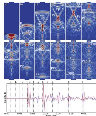
Figure 5: Left: Snapshots of the wavefield propagating through the cylinder with length 100 mm for a slice parallel to the y-z plane through the sample's center. The snapshots a) to l) correspond to times marked in the seismograms below with vertical dashed lines. Laboratory and synthetic data are colored in red and blue, respectively. Top: Mesh of a cylinder with a diameter of 40 mm and a length of 50 mm.
