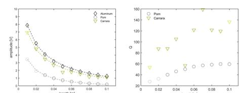
Figure 3: Amplitude decay with increasing sample length. Symbols show first minima, dashed lines are calculated from eq. (1) based on the parameters provided in Table 2.
