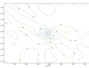
Figure 6: Contour plot of the misfit between computed and measured waveforms as a function of P-wave velocity V<sub>p</sub> and S-wave velocity V<sub>s</sub> for Alu. The small, blue dots represent the points where the misfit was actually calculated. The misfit surface was interpolated on a grid with equal spacing of 25 m/s. The contour interval is 5.
