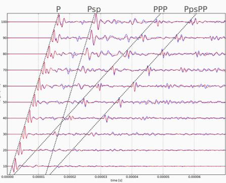
Figure 9: True seismograms (red) measured for ten rock samples of Carrara marble of different length, compared to synthetic seismograms (blue) computed with SPEC2FEM 3D using a quality factor of Q<sub>μ</sub> = 22 (Q<sub>p</sub> = 50; ignoring samples longer than 70 mm).
