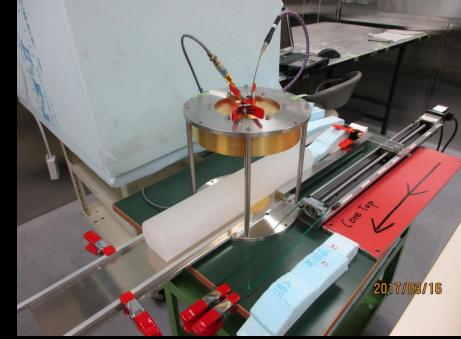
Figure 2. Firn core in the open resonator.
