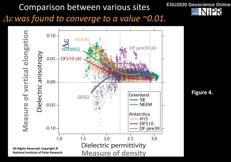
Density-anisotropy relation also strongly depends on sites.  $\Delta \epsilon$  was found to converge to a value of ~0.01. This fact means that <u>vertical compression causes vertically elongated geometry</u>.
