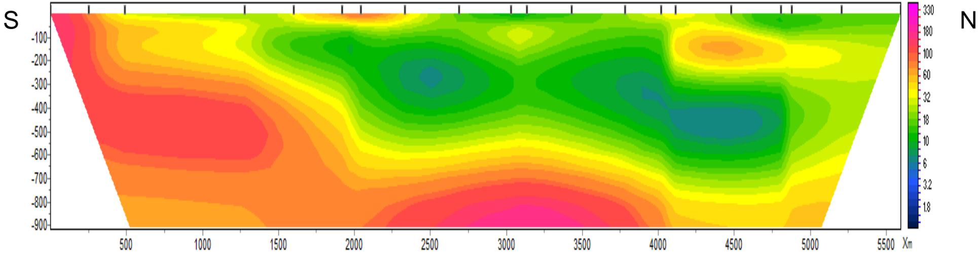
Electrical resistivity Tomography after the inversion procedure with the ZondRes2D software
