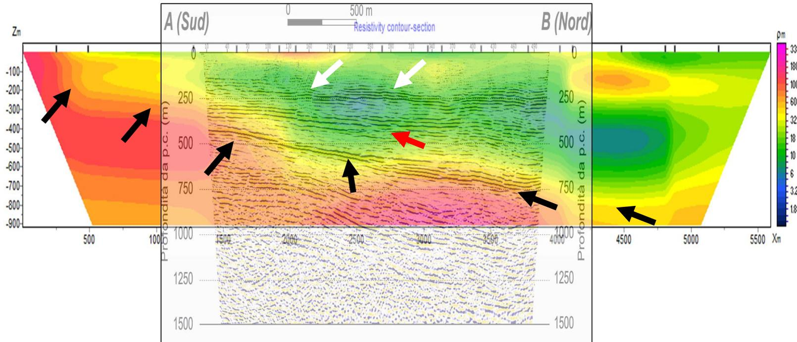
The joint interpretation of DERT and seismic data allowed to reconstruct the 'local' stratigraphic-depositional evolution until a depth of about 1 km, and to highlight the occurrence of a sin-depositional Quaternary tectonic tilting associated to the growth of a fault-propagation fold.
