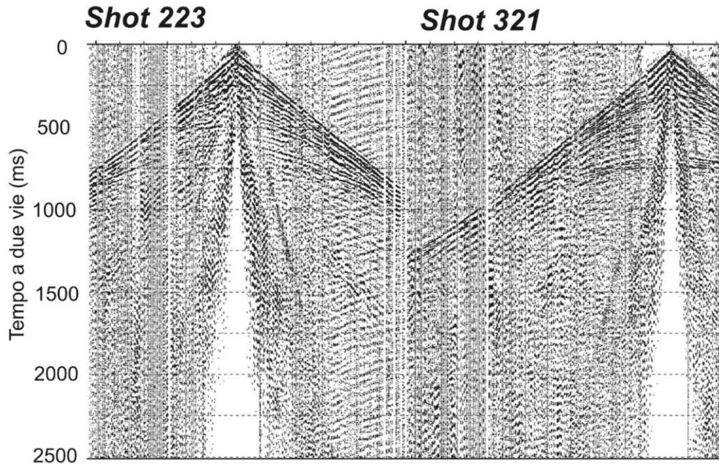
Example of two energizations after ground force correlation. Note on shot 223, the periodic noise induced by the passage of cars at the end of the line (right), which does not, however, mask the strong reflection at TWT at 750 s. Shot 321 records only random noise.
