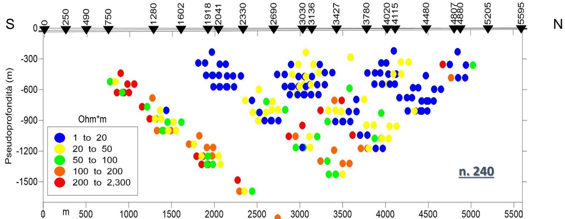
Distribution of the apparent electrical resistivity values obtained from the elaborated acquired data
