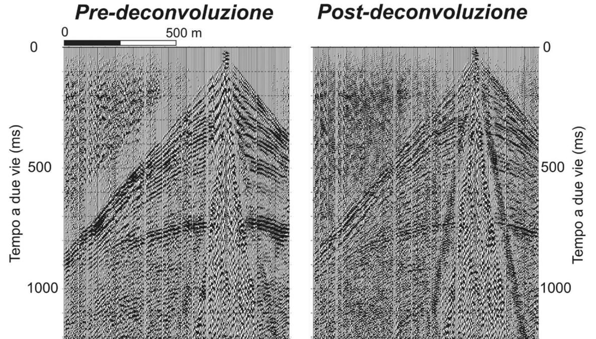
Example of a shot where a deconvolution has been applied. On the right you can see the considerable increase in the vertical resolution of the reflections produced by the algorithm.
