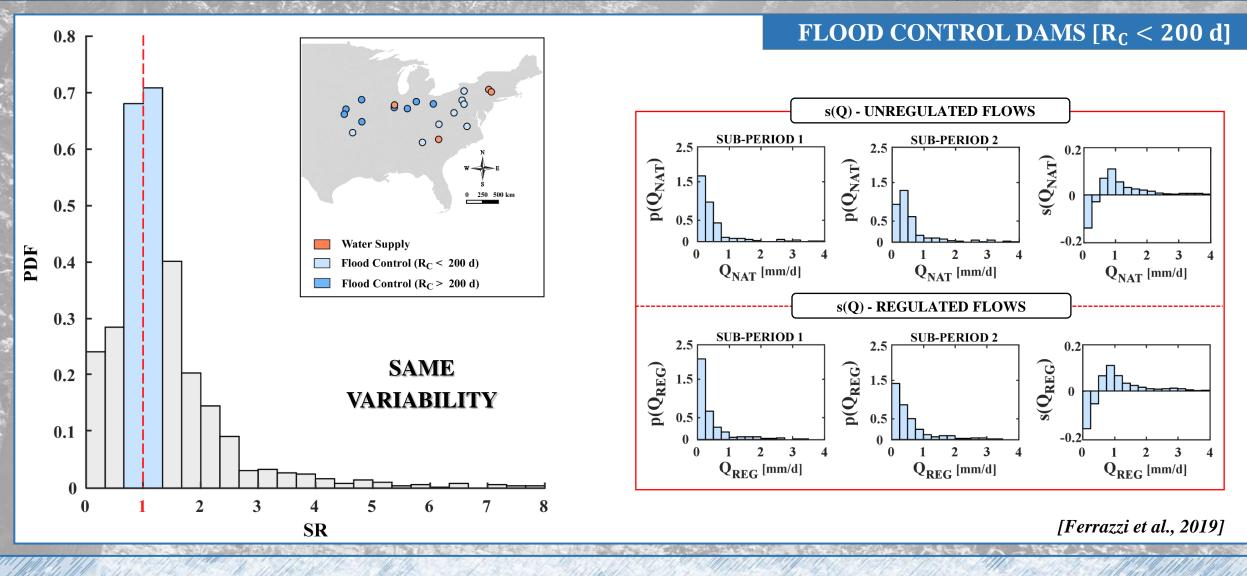
LOW REGULATION CAPACITY DAMS LEAVE UNALTERED STREAMFLOW FLUCTUATIONS
