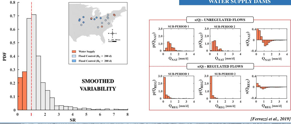
WATER SUPPLY SMOOTHS FLUCTUATIONS BY NARROWING THE SPECTRUM OF FLOWS
