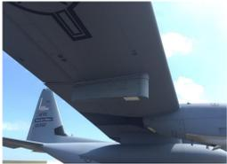
Radiometer under the wing of the aircraft NOAA
