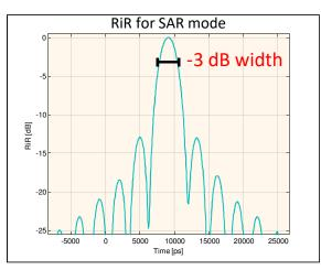
Requirement on -3 dB width: 0.394 m < -3 dB width < 0.436 m.
