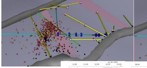
Events occurred whenever the fracture opening pressure was exceeded, with similar rate
