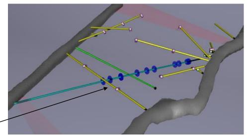
The majority of events occurred during the periodic pumping tests, the seismic clouds extend ca. 5 m radially from the stimulated interval
