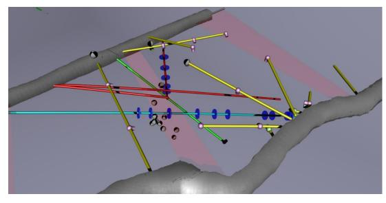
Systematic FMs with N-S to NW-SE Ρ trending nodal planes (that differ in orientation compared to the cluster elongation), dominated by shear faulting CLVD (+) (green in Hudson plot, on right)
