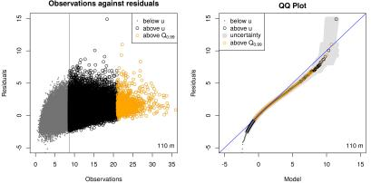
Legendre model diagnostics: censoring threshold  $u = 8.65 \text{ ms}^{-1}$  for MLE at 50 % quantile
