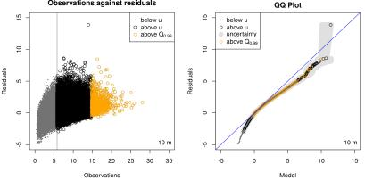
Legendre model diagnostics: censoring threshold  $u = 5.79 \text{ ms}^{-1}$  for MLE at 50 % quantile
