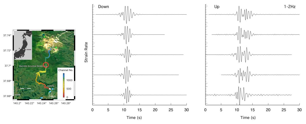
Waveform depends on the direction and the type of vehicle
