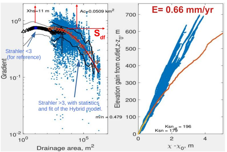
We fit the slope-area median with the hybrid model and obtain  $A_c$ ,  $S_{df}$  and  $\theta$ .
