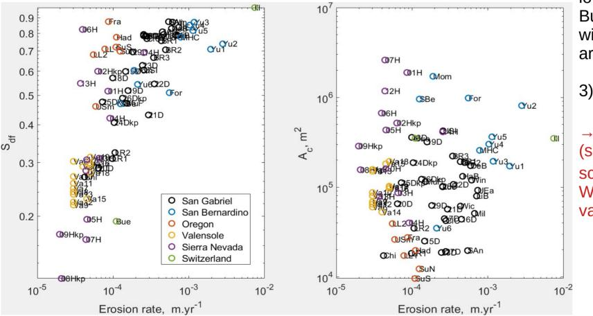
2) Sdf can be pretty low ~0.2 (10°) But not inconsistent with DF angle of arrest.
