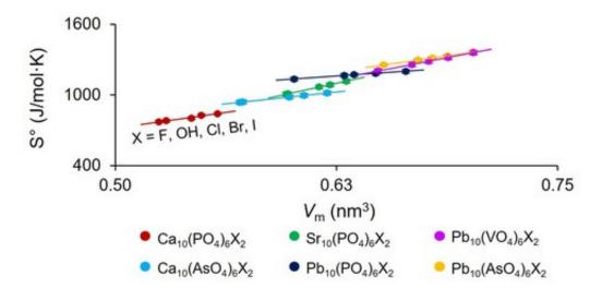
**Fig. 1** Standard entropy ( $S^\circ$ ) vs. formula unit volume ( $V_m$ )for selected apatite subgroups. Errors bars are within the marker.
