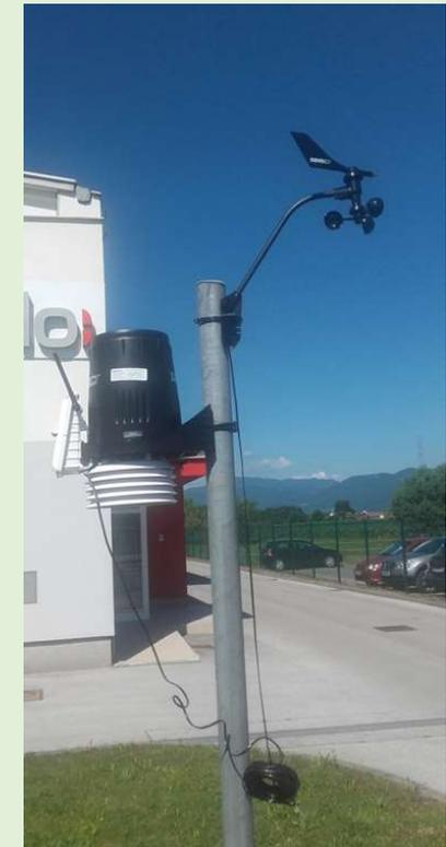
measurements of air temperature and relative humidity inside + meteorological station outside
