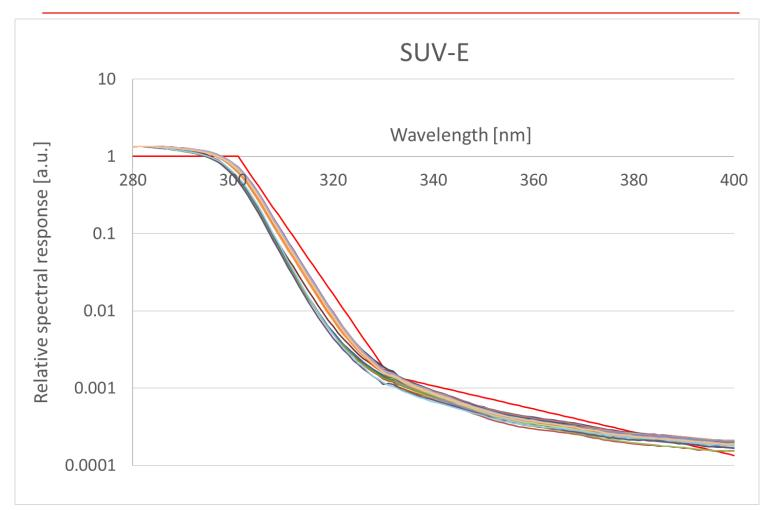
Lab. response curves of production SUV-E and CIE curve
