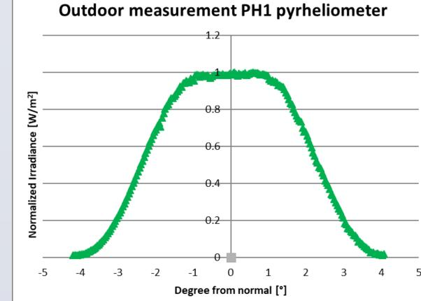
The PH1 pyrheliometer angular response or effective penumbra function was measured in the lab and outside. In the lab a lamp and an angle indicator was used. Outside the PH1 was pointed to a point where the sun would pass at a later moment and then measured over time. The measured slope angle, opening half angle and limit angle [6] are in good agreement with the expected values of  $1^{\circ}$ , 2.5° and 4°.
