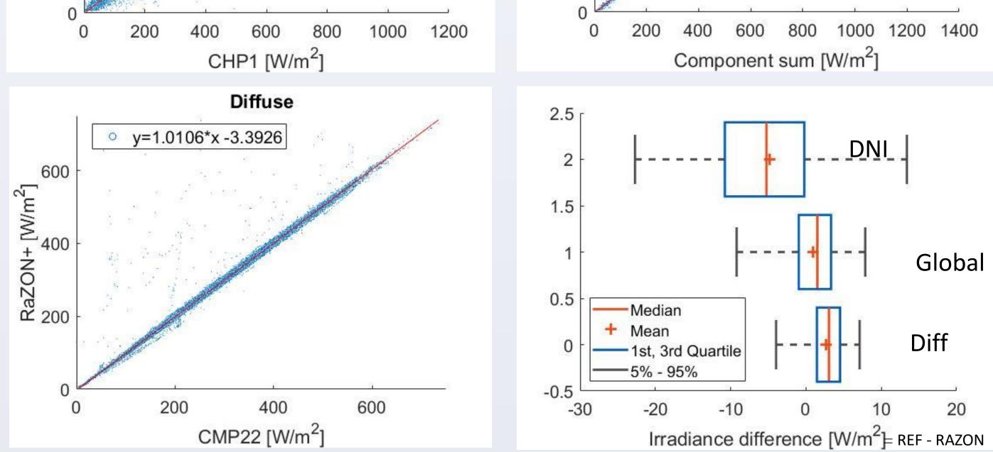
The comparison of the RaZON+, with the reference system is shown above.
