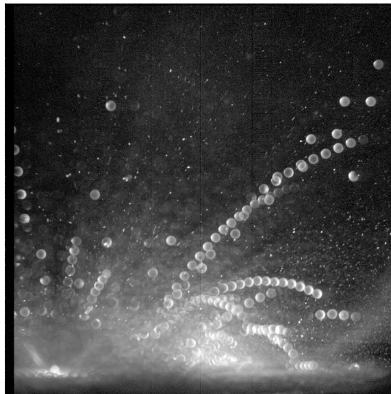
Figure 4: Trajectories of ejecta measured for 5mm projectile launched at 1.06km/s into 5mm spheres.
