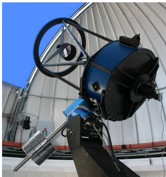
Figure 1: The new robotic 0.6m TRAPPIST telescope installed by the Liège University (Belgium) in La Silla observatory (ESO, Chile).
