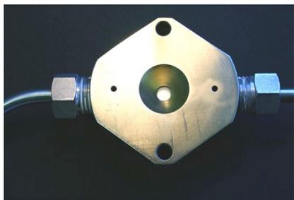
Figure 2. Photograph of the fluid pressure cell.
