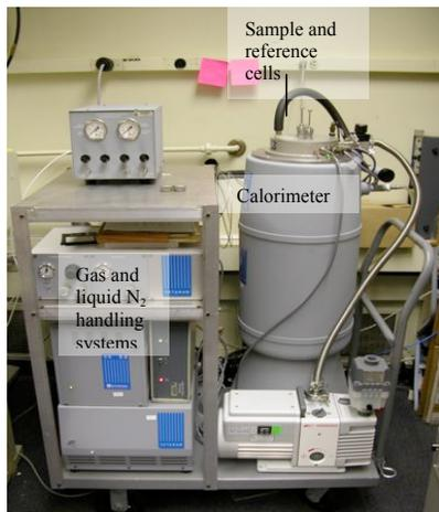
Figure 1: Photograph of the Setaram BT2.15 Calvet calorimeter.
