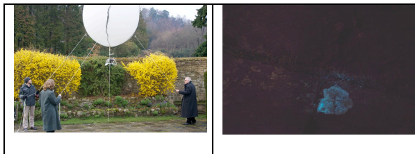
Figure 4. Aerobot test controlling the balloon with the picavet with the instrument payload (upper) and result of imaging the fluorescence of blue-green algae with a 30s exposure.
