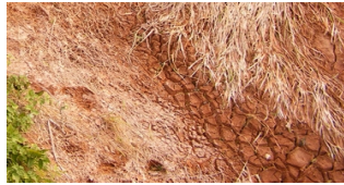
Fig. 4. Sludged red-mud surface with white gypsum remnant dust cover at Boba bridgehead measuring point.
