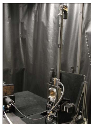
Figure 1. Bloomsburg University Goniometer (BUG) setup
