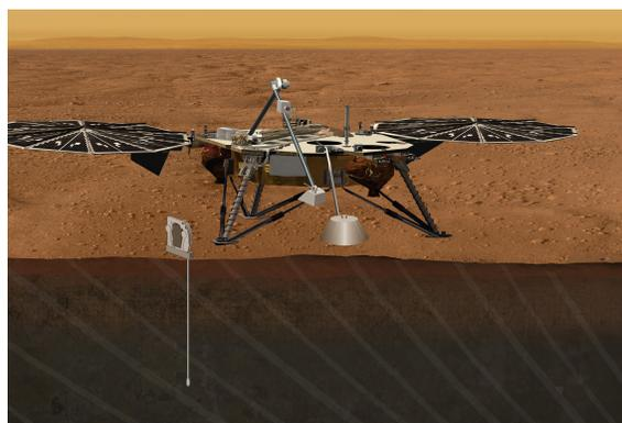
Figure 1: Conceptual view of the GEMS lander including the deployed seismometer and heat flow probe (HP<sup>3</sup>).
