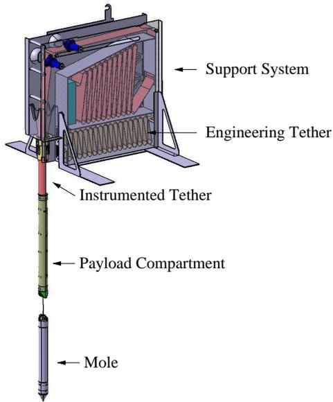
Figure 2: Schematics of the HP<sup>3</sup> instrument showing the functional subsystems.
