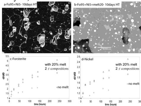
**Fig2:** (a & b) SEM images showing the evolution of the microstructures between samples without (a) and with silicate melt (b). Note that the scale is one order of magnitude different between the two pictures. (c & d) Evolution of the grain size with time and sample compositions. In both phases, grain growth is faster in the presence of silicate melt. Finally, note the influence of the composition of the silicate melt on grain growth.
