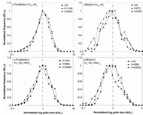
**Fig.1:** Normalized grain size distribution as a function of annealing time and sample compositions. Note that a steady-state distribution is reached for both phases Fo and Ni in dry (a & c) and wet conditions (b & d).
