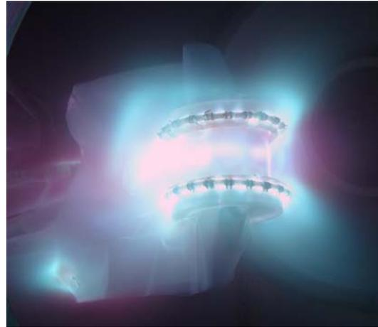
Figure 1: Plasma generated by surface discharge using two coils placed around magnetic dipole.
