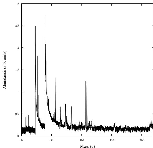
Figure 1: A sum spectrum of 32 impact ionisation mass spectra of anorthite grains which impacted at velocities of between 5 and 6 km s<sup>-1</sup> onto the LAMA laboratory model.
