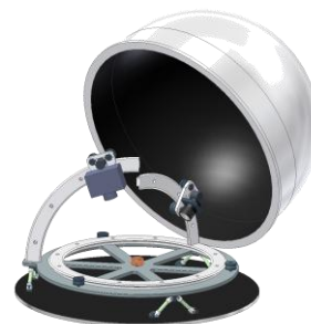
Figure 3: CAD model of the goniometer, showing the surrounding cold-shield, solar source and detector mounted on computer-controlled moveable arms. All of this would be placed in a low-pressure vacuum chamber to simulate the lunar environment.
