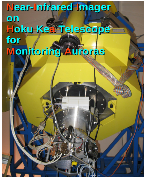
Figure 2: The NIIHAMA camera as attached to the Cassegrain port of the Hōkū Ke‘a telescope (during the balancing test in November 2010).
