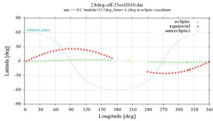
Figure 1: Scan plane for the zodiacal-light observation. Green and red symbols are the same but with different (ecliptic or equatorial) projection.
