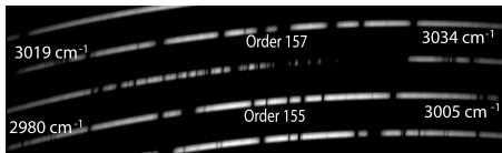
Figure 1. Orders 155 and 157 from the L3 setting of iSHELL. These orders contain absorption lines of the P- and R-branches of CH 4 along with water. These two orders were isolated, cleaned of hot and dark pixels, and straightened.
