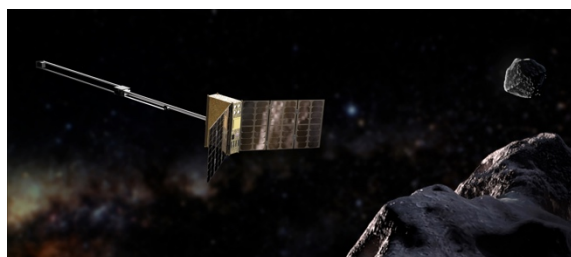
Figure 1: APEX Cubesat rendering, with deployed arrays and magnetometer boom. Image credit: Tomi Kärkkäinen / Reaktor Space Lab
