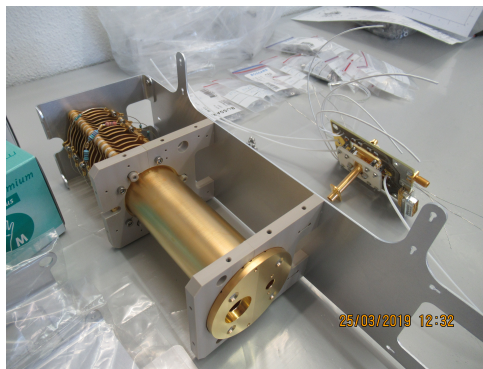
Figure 2: Photograph of the new reflectron-time-of-flight mass spectrometer under assembly.
