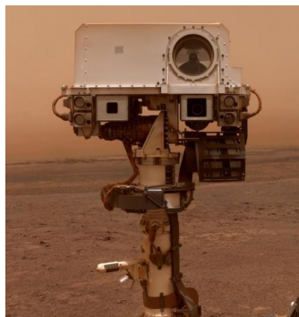
Figure 1: Curiosity rover with REMS-H device visible on the mast below wind sensor. Credit: NASA
