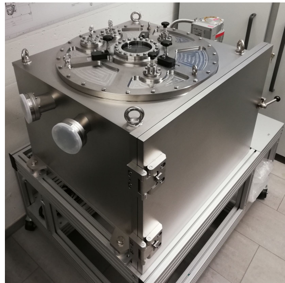
Figure 1: The SCITEAS-2 simulation chamber that will be used in our sublimation experiments.
