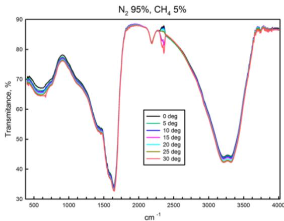
Figure 2: Transmittance spectra of the N<sub>2</sub>-CH<sub>4</sub> (95:5) obtained at different angles. (NB: contribution from gaseous CO<sub>2</sub> from the FTIR spectrometer purge can be seen around 680, 2300 and 3400-3800 cm<sup>-1</sup>).
