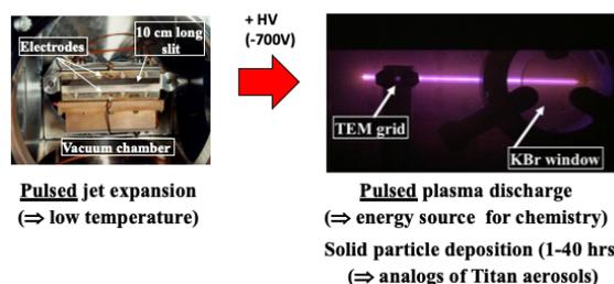
Figure 1: Pictures of the THS PDN (*left*) and plasma discharge during sample deposition (*right*).
