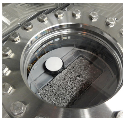
Figure 1: Picture of a sample made of micrometer-sized particles of water ice intimately mixed with lunar regolith simulant (JSC1-AF) and carbon black particles sublimating in vacuum seen through the window of the SCITEAS experiment. The diameter of the window is 16 centimeters. The white round object is a standard reflectance target.
