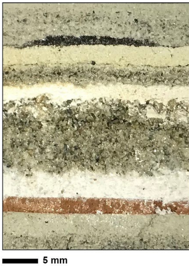
Fig. 3: Micro-layered samples composed of ground rocks and single minerals with different grain sizes.
