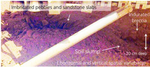
Figure 4: Area beneath the lander with struts, retrorockets, and excavated pits (10-20 cm deep). Steep pit walls (> angle of repose) indicate cemented duricrust.
